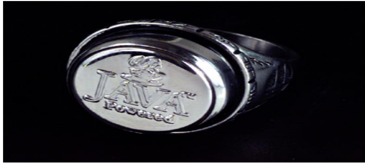
FIG: The Java Ring can be programmed to give you access to every door and device.
